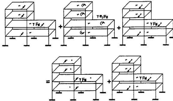
Figure 5. Second load case of Figure 4 as a combination of steps 1 and 2 of the new approach
