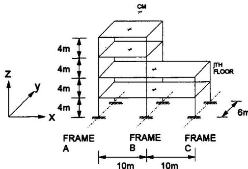
Figure 6. Example building (After Tso, 1990)
