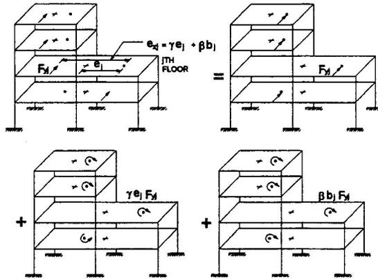
Figure 4. Conceptual explanation of the new approach
